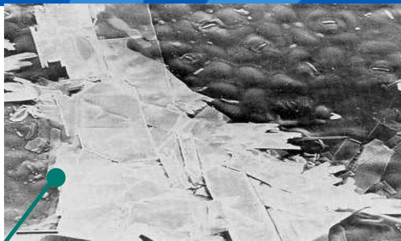
Strong amount of metal residues caused by oxides applications.
